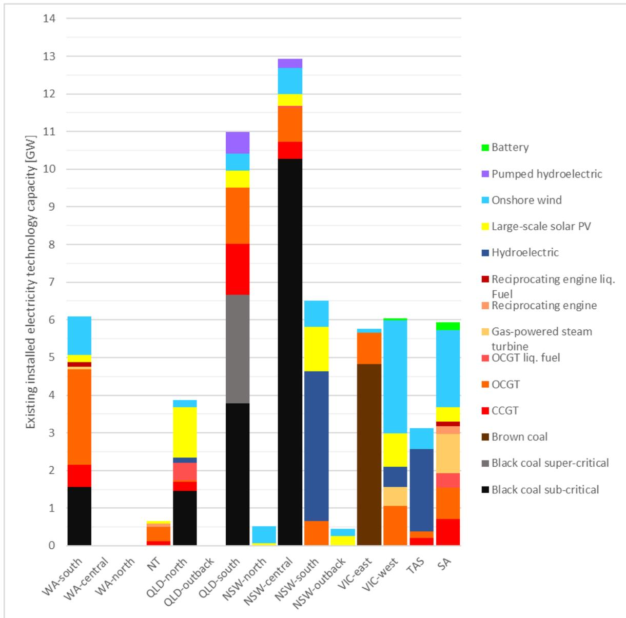
Figure 59 | Maximum yearly installed capacity of currently existing electricity technologies, based on the expected retirement year listed in the various planning studies.<sup>[2,3,4]</sup>
