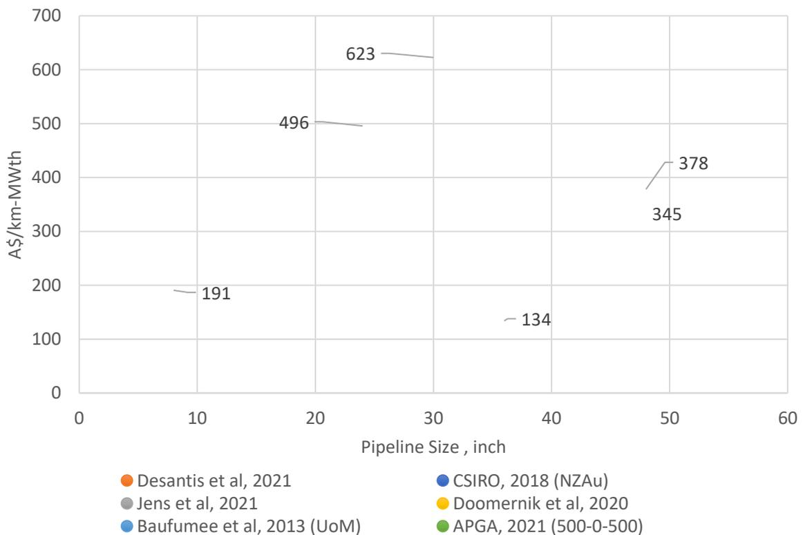
The above capital cost compare based the size of pipeline in AU\$/in/km in Table 71. The result shows that the hydrogen pipeline cost is in range of AU\$108k/in-km to AU\$125 k/in-km. As the majority of hydrogen pipeline is used for transferring hydrogen to the ports, the cost of pipeline was adjusted to 280 AU\$/MW-km for the maximum size of 56 inch using Jens et al.<sup>[17]</sup>
