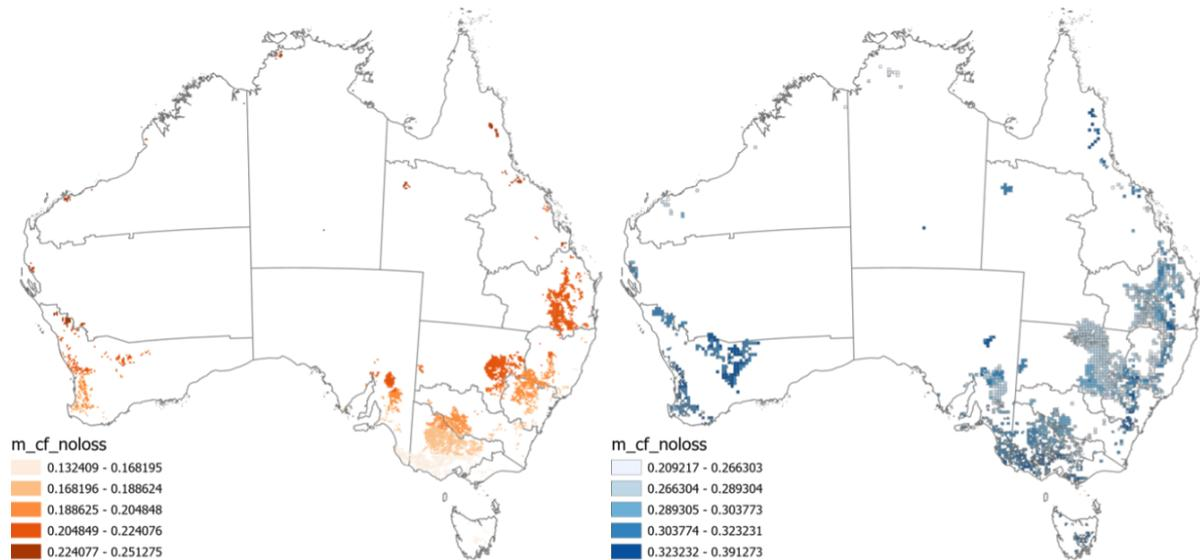
**Figure 48 | Location and capacity factors of projects in the solar PV (7.1 TW) and onshore wind (1.9 TW) export supply curves after applying all filters in Table 31 (note that m\_cf\_noloss represents the mean capacity factor with no losses).**
