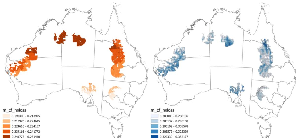
Figure 49 | Location and capacity factors of projects in the offshore wind domestic (2.4 TW) and export (0.2 TW) supply curves after applying all filters in Table 31 (note that m\_cf\_noloss represents the mean capacity factor with no losses).
