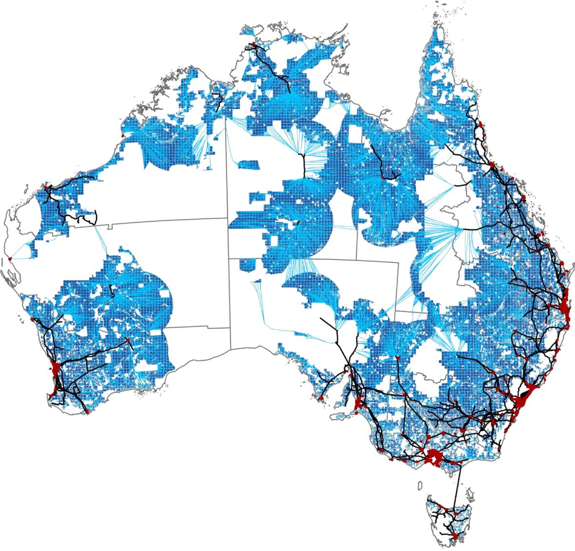
Figure 87 | Map of all possible bulk transmission lines (orange) connecting the point of intersection between spur lines (light blue) and existing transmission lines (black), and final load/transmission destinations (red).
