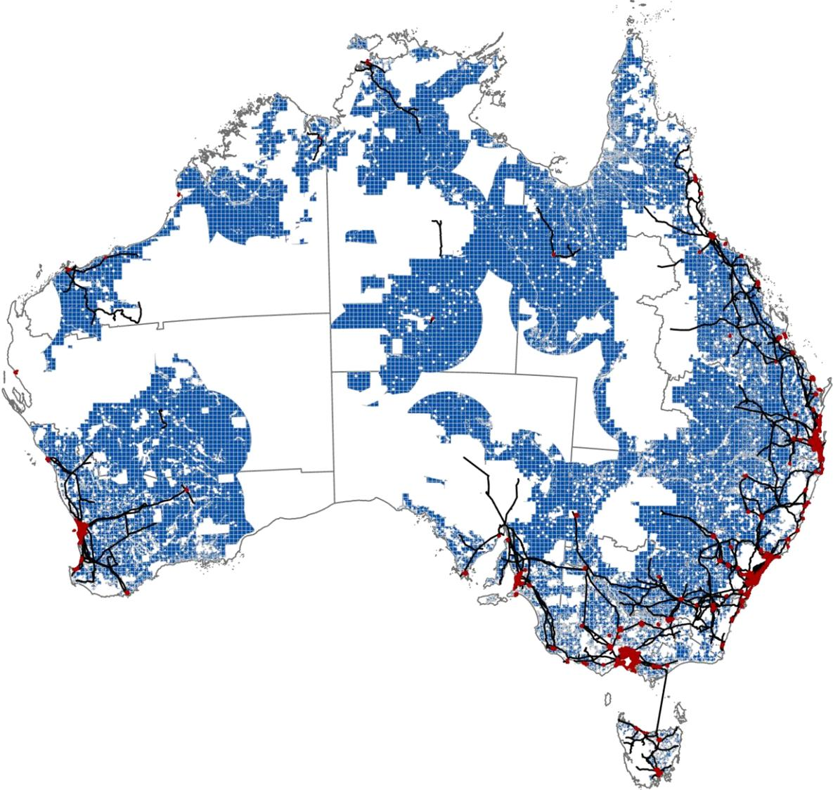
Figure 86 | Map of spur lines (light blue) connecting all potential domestic wind projects (dark blue) with existing transmission lines (black), and final load/transmission destinations (red).
