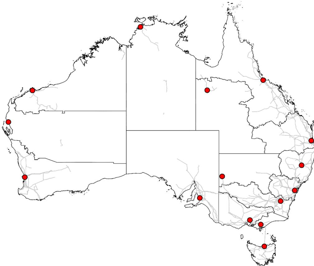
To model inter-regional electricity transfer, each region was assigned a node or ‘reference point’ through which electricity can be transferred to and from other regions. Of course, in practice electricity transfer may occur through multiple lines. Therefore, for this approximation to be reasonable, the reference points must be chosen to represent the bulk of the electricity transfer between the regions.
