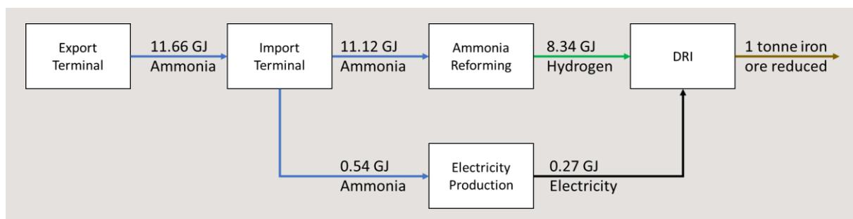
Figure 6 | Flowchart of energy export transformation for Aluminium Production and the impact of E+ Onshoring. Incorporates efficiencies of 75% of ammonia reforming and 50% of ammonia to power.<sup>[9,11]</sup>
